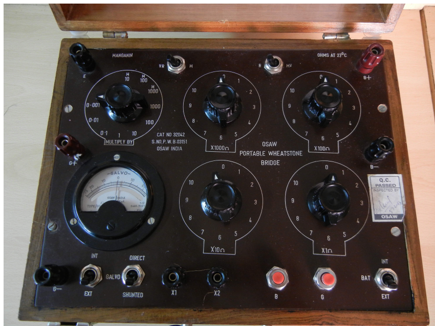
Figure 1.2: A wheatstone bridge setup.
