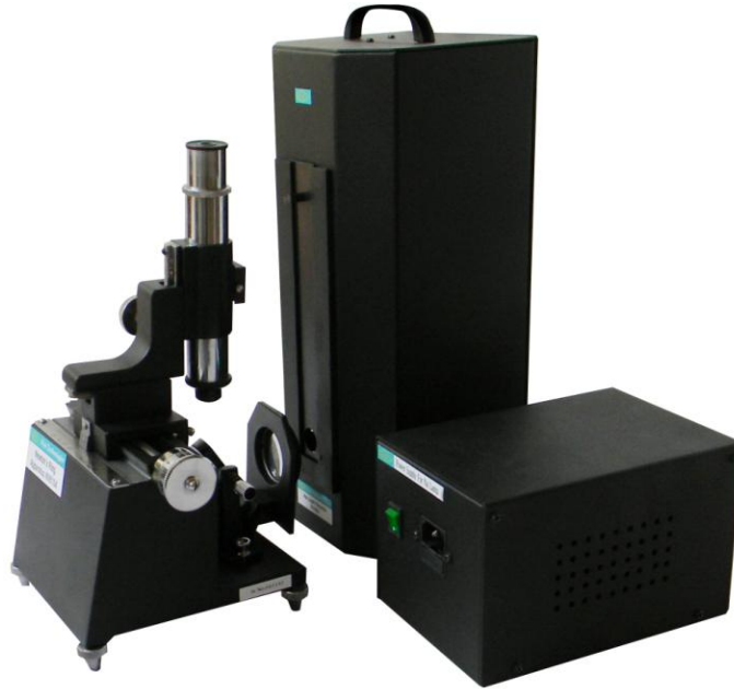
Figure 6.1: Experimental setup of Newton's ring
